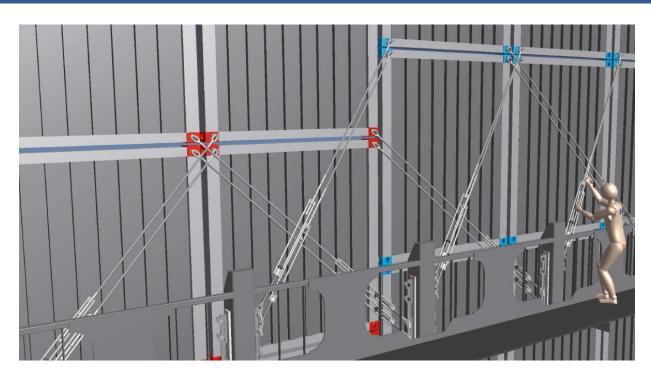
A Unique New Lashing Method to combine External & Internal Lashing and any Size (8'.6" to 9'.6") Containers with a Single Type/Size of Bar!
